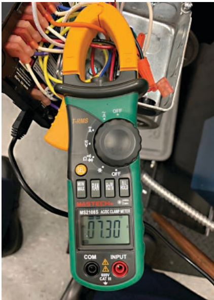
Figure 11-3: Locked rotor amperage
