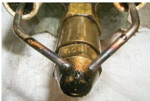
Figure 12-3: Electrodes showing excessive wear
