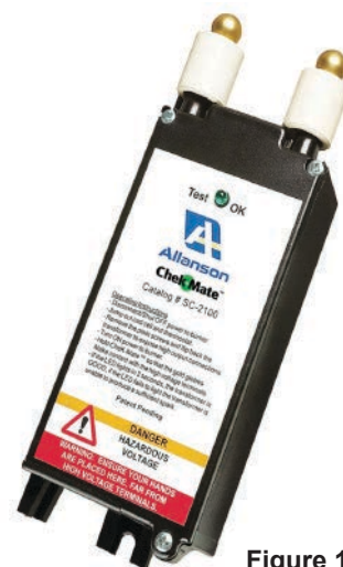
Figure 12-5: Instrument to test both transformers and ignitors
