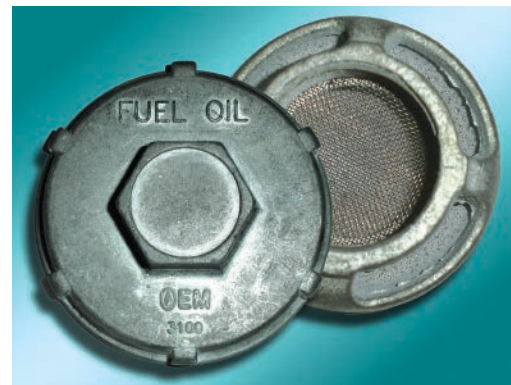
Figure 3-17: Fill pipe should be clearly marked "Fuel Oil" and the vent cap should contain an insect screen.
