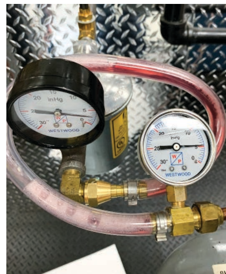
Figure 7-25: Suction line analyzer showing air bubbles in the fuel
