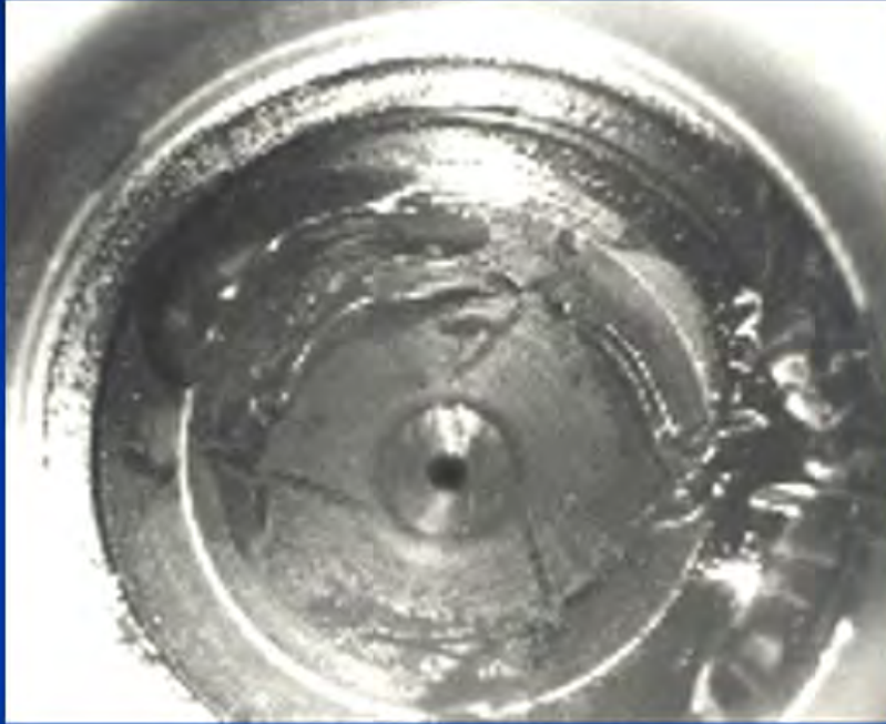
Iron oxide contamination build up in the standard nozzle
