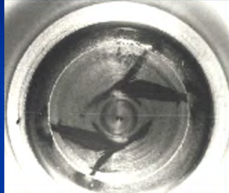
Dark streaks on the Del-O-Flo show a discoloration from sand with no contamination build up
