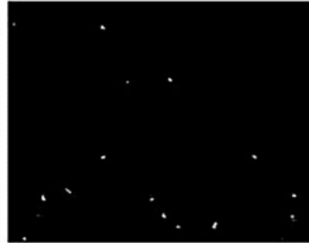
Diesel fuel at cloud point A few wax crystals appear instantaneously
