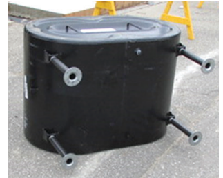
Fig. 1 – General photo of assembled tank and slab before anchoring - Note all photos are of ½ size horizontal obrounds tested, but the hold down methods apply to vertical obrounds.
