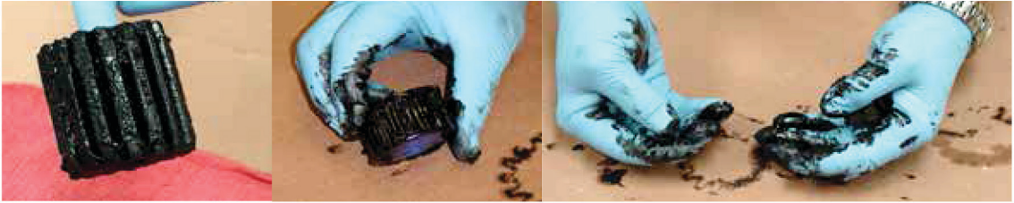
If a sludge problem persists, fuel testing/treatment and tank cleaning/replacement should be considered.
