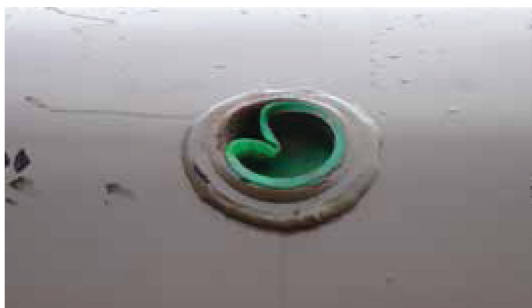
Even with plugs in place, tanks can accumulate water while in storage.
